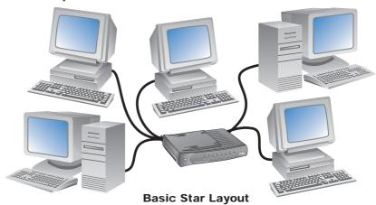
Installation is simple, inexpensive, and fast because of the flexible cable and the modular connector. The number of nodes you can connect to a hub is determined by the hub. There is a limit to the number of nodes you can add on a network (a maximum of 1024 nodes.). The star layout becomes a workgroup and can operate independently or can be connected to other workgroups.
